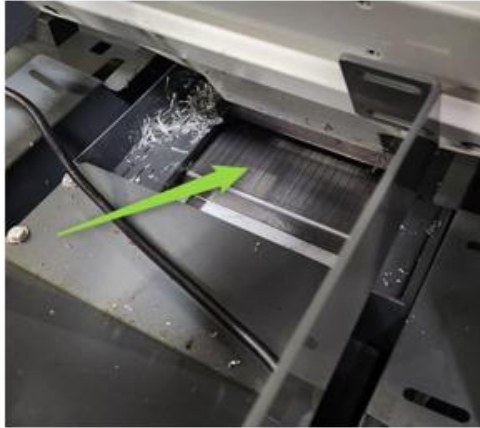
Wire Brushes wipe chips from Coolant Filter Box
