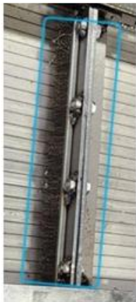
Wire Brushes wipe chips from Coolant Filter Box
